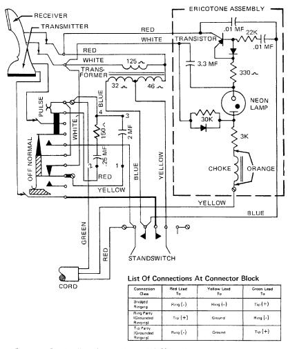
Figure 1.1. Ericofon Wiring Diagram Number 520533, for Manual and Dial Base Models with Ericotone (Models 52L and 52J).
